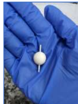
Figure 1b: Sample sealed source for activation. The stems help in the preparation of the source.
